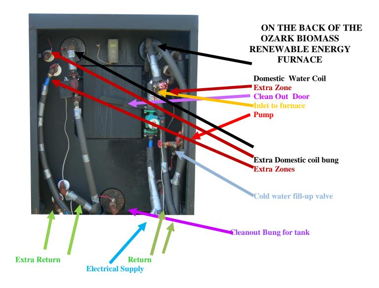
While furnace is in use valve above pump should be opened, valve on return line should be opened. The cold water fill up valve should be shut except while filling up furnace tank.
