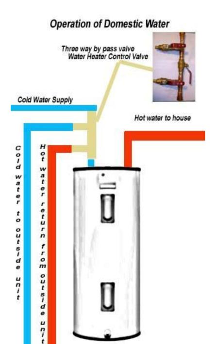
When side valves are opened and middle valve is shut your outside furnace will heat your water. Reverse for water heater only.
